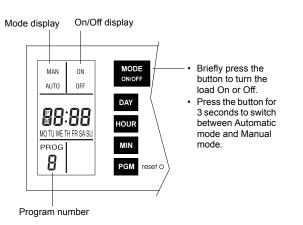
At power-on, 0:00 will flash. Otherwise, press **reset** using a paper clip. If the display is blank, verify the power supply.
