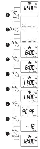
NOTE: The timer automatically returns to its normal display if you do not press any button for 60 seconds.
