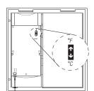
Replace the front part of the thermostat on the base and secure it in place with the screw.
