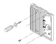
Set the switch at the back of the removable part of the thermostat to °C or °F.
