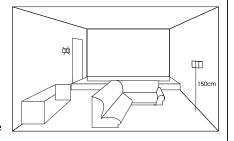
Fasten securely the thermostat to the wall with the two (2) screws.
