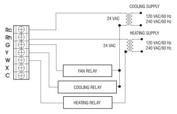
WARNING: Remove jumper between terminals Rh and Rc: Both 24 volts returns of the transformers must be connected together in order to have the fan working with the heating and the cooling system. \*Otherwise, the fan will only work with the cooling system.
