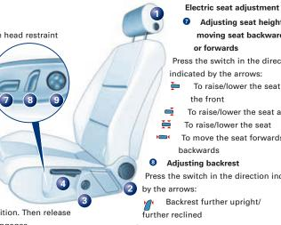
Adjusting seat height and moving seat backwards or forwards Press the switch in the direction indicated by the arrows: To raise/lower the seat at the front To raise/lower the seat at the rear To raise/lower the seat To move the seat forwards/ backwards 8 Adjusting backrest Press the switch in the direction indicated
