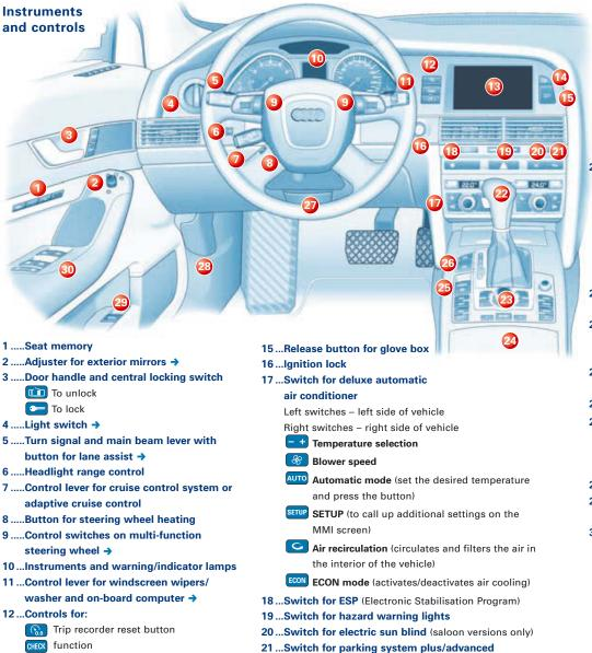
The parking aid is activated automatically when reverse gear is engaged. Press this button to activate the system when moving forwards.
