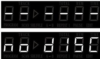
Turn the power on by pressing the key on the rear panel near the IEC mains socket. The player will start searching for a disc. If there is already a disc in the tray, the total time and number of tracks will be displayed; if not "NO DISC" will be displayed.
