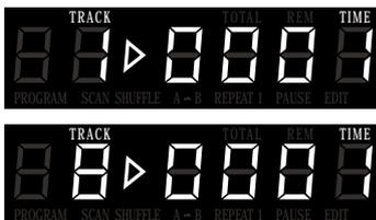
To play the disc, press the PLAY key; playback will start from the first track of the CD or from the first track selected in the program. If you wish to start playback from another track, this can be done by either selecting sequentially using the PREVIOUS and NEXT keys on the front panel or directly from the remote control using the numerical keypad. The playback symbol, the current track number and the elapsed track time will appear on the display.
