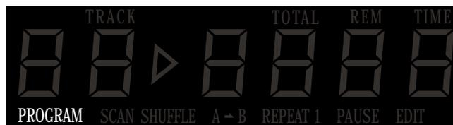
**PROGRAM** Flashes when programming is in progress. Glows steady after programming, until program is deleted.
