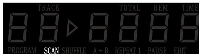
**SCAN** Indicates the activation of automatic CD tracks' scanning.
