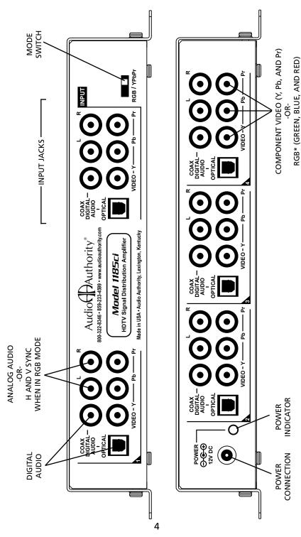
\* IN RGB mode, be sure to connect H and V to the analog left and right audio jacks.
