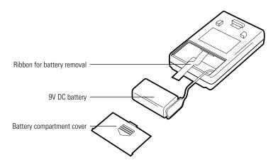
**Note:** To avoid possible damage due to leakage, the batteries should be removed if the PRO 88W will not be used for a long time.
