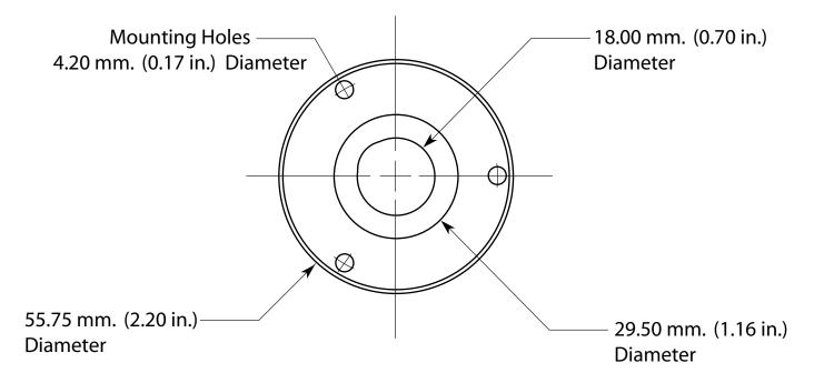
This template is shown actual size. To create a template to mount this baseplate to your turntable, print this page at 100%. Check the dimensions on the printed page BEFORE drilling any holes in your armboard.
