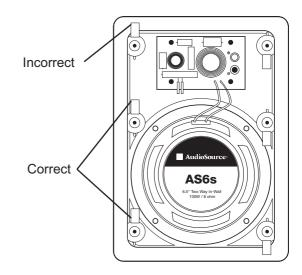
With the grill removed, place the speaker in the wall opening. Make sure that the speaker wire is not hanging against the speaker where it can vibrate and rattle as the speaker reproduces your music.
