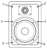
Tighten all six of the mounting screws in the same manner until the speaker is properly aligned and held tight to the wall surface. *Caution:* Do not over tighten!
