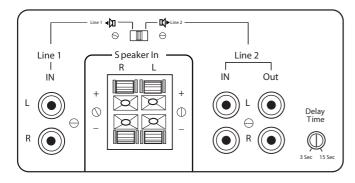
There are a total of 4 RCA inputs on the back panel of the AMP200. These RCA inputs are labelled as "Line 1 Input" and "Line 2 Input". They are also designated with an "R" or an "L" as Right channel or Left Channel inputs respectively.
