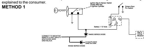
To connect to the key in sensor as shown in method 1:
