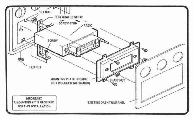
Important-This installation is designed for 1984 and older U.S. made Ford cars, trucks, and vans. For newer vehicles, an installation kit may be required. See Kit Listing on Page 2 of this manual or refer to the in-store chart.
