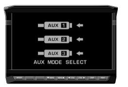
IF there is no button presed within 5 sec or 「DISP」 button is pressed, mode is switched back to the previous mode.
