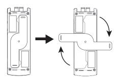
1. Before using the tuner, rotate the support bar clockwise. Make certain the unit is stable before extending and rotating the antenna rods.
