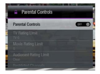
Use the  $\blacktriangleright$  (right arrow) key to highlight the parental on/off control and press OK to enable it or disable it. Once enabled, press the OK key and you will be prompted to create a PIN (Personal Identification Number) as shown in the following screen:
