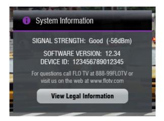
This screen tells you the signal strength of the FLO TV signal. If you are having reception problems, go to this page to see if the FLO TV signal is available at your location. (Note: The Device ID will be different from the above screen, which is for reference only.)
