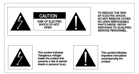
• To avoid electric shock, never touch the inside of the LCD TV. Only qualified technicians should open the case of the LCD TV
