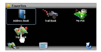
If no trip exist, the system will display "There are no saved trips. Add?". Press the green check mark button to go directly to the "Enter Name of Trip" screen and continue with Step 4. If trips exist, continue to step 2.
