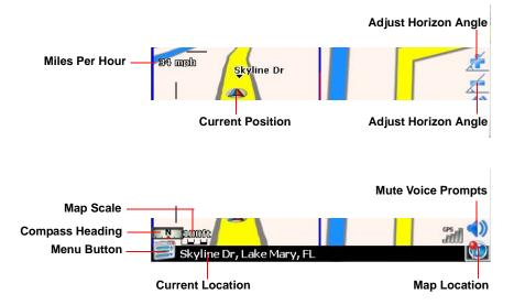
On the left, additional information, including the map scale and compass orientation (N, S, E, W) is displayed.
