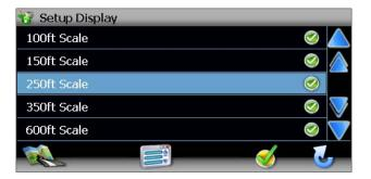
10. Press the green check mark next to each scale setting to make your trail visible at that scale.
