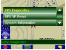
The GPS diagnostic displays the number of GPS satellites currently in view and how many are currently being used. The GPS satellite time is displayed (UTC) and so is the latitude and longitude determined from GPS.
