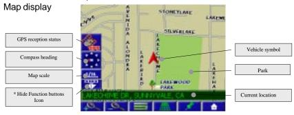
The GPS symbol will change colors indicating the strength of the signal. The GPS symbol colors mean:
