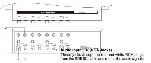
to the SDB (Signal Distribution Box) from the source component (Example VCP, DVD etc.). Use the SDBSC cable.
