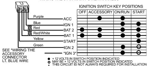
WIRING THE 6 PIN MAIN POWER HARNESS
