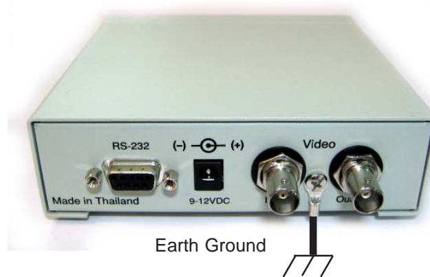
Figure 5 : VSI-Pro Max Earth Grounding Connection
