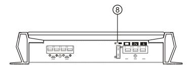
Off to a normal operating range. If activated by an overload condition, the source of the overload must be found and corrected to resume operation of the amplifier. Most overload conditions are caused by mis-wiring or operation into incorrect speaker loads. Re-check all wiring and connections if this situation occurs and correct as necessary.
