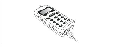
Insert the travel charger connector into the battery charging socket at the bottom of the handset. Make sure the flash mark on the connector faces upward when you insert it.
