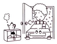
When the moisture condensation occurs inside of the VCP, NEVER insert the cassette into the cassette compartment. Remove the cassette if loaded, by pressing the STOP/EJECT key. Only operate the VCP after moisture condensation has completely dried out. Normally, it takes about two hours.
