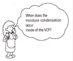
If the VCP is moved from a cold place to heated place, or the temperature of the VCP's surroundings goes up due to room heat being switched on. Or if the VCP suddenly moved from an air conditioned room to place with a of high degree of humidity in summer. This may cause the dew indicator light to light up. Do not use the VCP in this condition.
