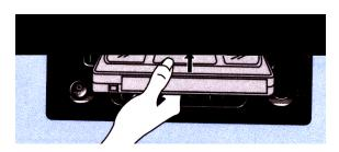
Upon inserting the cassette, the power turns on even if the power was off as long as the DC power cord is plugged in. Press the STOP/EJECT key twice on the VCP (in the PLAYBACK mode). This first press will stop the
