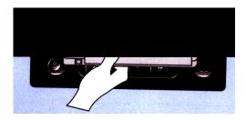
When you press the STOP/EJECT key even if the power is off, the cassette will be ejected.
