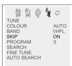
5 Press the TUNE button to close the menu. When you use the P+/buttons to select channel, this channel will be skipped. However, you can still use the PROGRAM NUMBER buttons to select the skipped channel numbers.
