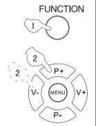
2 Press the P+/- buttons to select "CHILD LOCK" and press the V-/+ buttons to turn CHILD LOCK function "ON".
