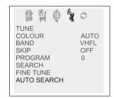
3 Press the V+ button to ensure automatic search function operates. All channels now playing program will be automatically preset in order. After the search has finished, the first program number will display on the screen.
