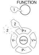
1 Press the FUNCTION button, the FUNCTION menu shown on the right display on the screen.
