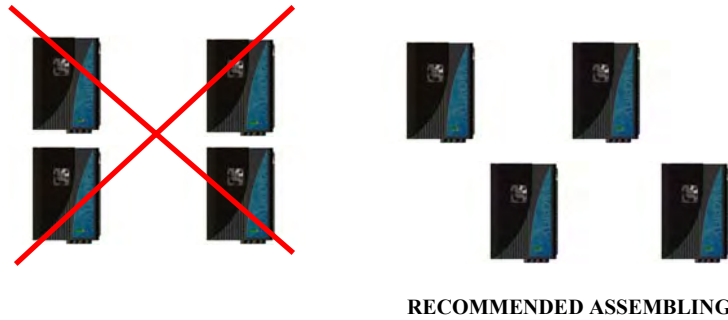
Fig.8 Recommended multi Aurora mounting
