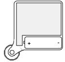
battery contacts. Replace the case cover and carefully tighten the screw. *Do not over-tighten the screw!* Test the transmitter to insure it arms and disarms the alarm.
