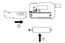
Note: Press the  $\square$  button two times when the battery compartment is empty, and then insert the new battery.
