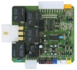
Auto Page remote start circuit boards maintain 30/45-ampere relays for reliable and long-lasting remote start performance.
