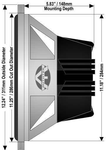
When designing an enclosure for this subwoofer, please ensure to leave atleast 2" of clearance from the back of the motor to the back of the enclousre.
