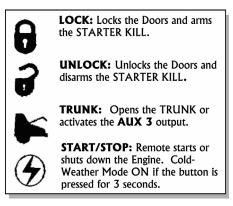
Note: Pressing the LOCK and UNLOCK buttons at the same time will activate the AUX 2 output. Remote-starting Your Vehicle
