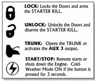
Pressing the LOCK and UNLOCK buttons simultaneously will activate the AUX 2 output.
