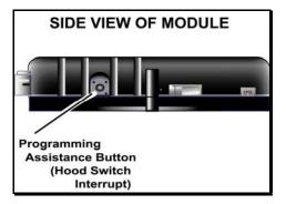
The PAB is located on the side of the module. This push button mimics the hood-pin switch in order to avoid having to get out of the vehicle and pressing the hood-pin switch. The PAB will work only when the hood is up.
