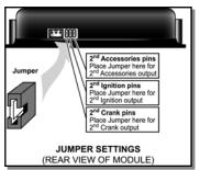
Remote car starters of this series are equipped with an on-board high-current programmable 5<sup>th</sup> relay that can be used to power a second ignition, accessory or crank wire. The unit uses 3 sets of pins; each set corresponds to a specific function of the output. In order to activate one of the three possible functions, you must place the jumper (supplied) on one of the three sets of pins and connect the 14 AWG wire to the second IGN. / ACC. / CRANK wire of the vehicle.
