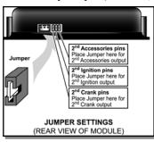
Remote car starters of this series are equipped with an on-board high-current programmable 5<sup>th</sup> relay that can be used to power a second ignition, accessory or crank wire. The unit uses 3 sets of pins; each set corresponds to a specific function of the output. In order to activate one of the three possible functions, you must place the jumper (supplied) on one of the three sets of pins and connect the 14 AWG wire to the second IGN. / ACC. / CRANK wire of the vehicle.
