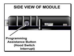
The PAB is located on the side of the module. This push button mimics the hood-pin switch in order to avoid having to get out of the vehicle and pressing the hood-pin switch. The PAB will work only when the hood is up.
