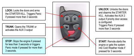
Note: Pressing the LOCK and UNLOCK buttons at the same time will activate the AUX 2 output.
