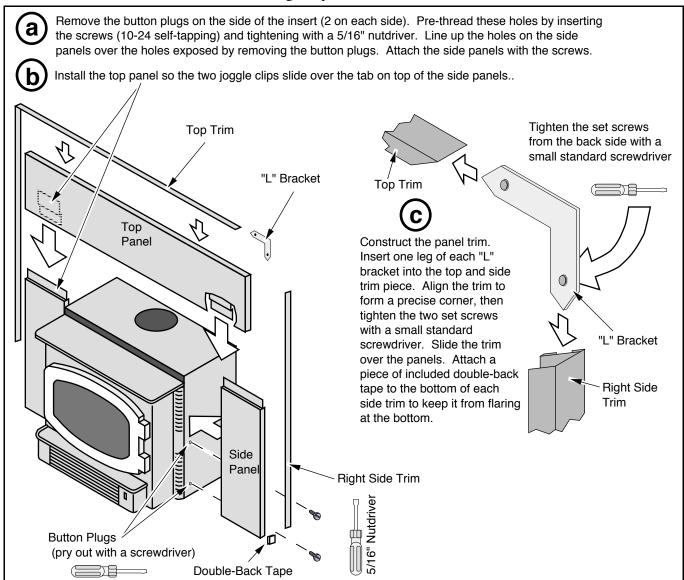
**NOTE**: Discard the insulation that comes with the surround panels (for wood stoves only). The panels must not form an air-tight seal against the fireplace.
