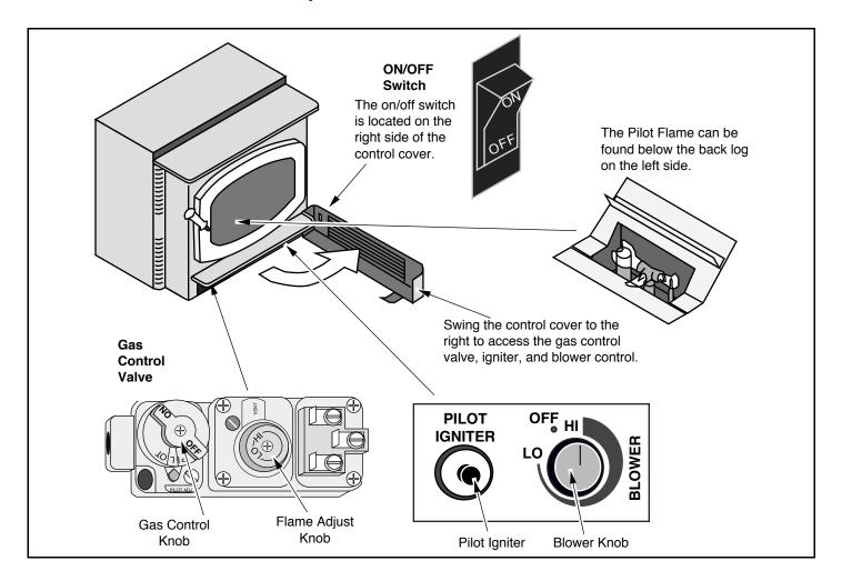
**Blower Knob** This knob controls the speed of the internal convection blower that pushes the
