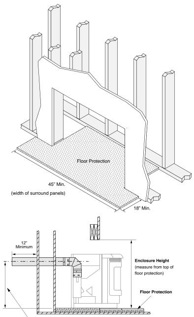
Place the stove on top of the floor protection and measure the center of the flue. This will determine the location of the wall thimble.
