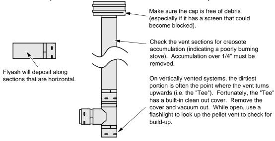
Warning: Whenever any portion of the pellet vent is disconnected, the joints must be sealed with RTV 500° F. silicone sealant.
