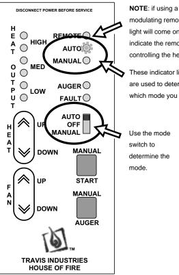
modulating remote, this light will come on to indicate the remote is controlling the heater.
