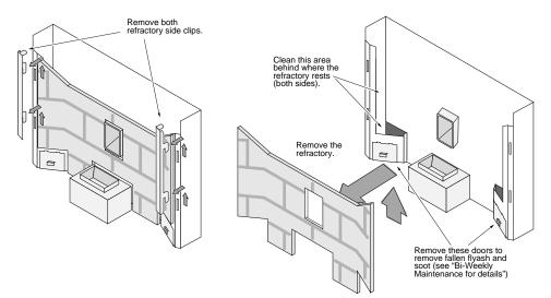
Clean the Horizontal Exhaust Duct (the stove must be cool and unplugged)
