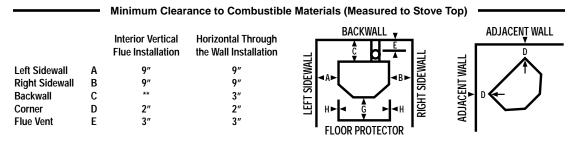
Maximum alcove depth 48 in/1220 mm, min ceiling height 60 in/1525 mm.
