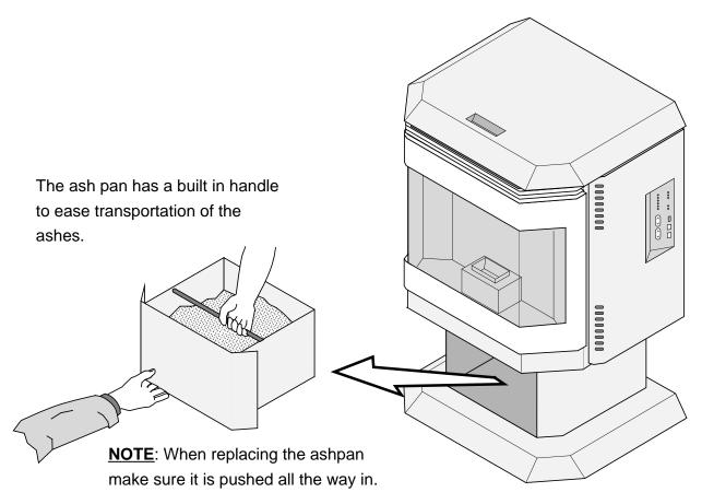
**Disposal of Ashes** – Ashes should be placed in a metal container with a tight fitting lid. The closed container of ashes should be placed on a noncombustible floor or on the ground, well away from all combustible materials, pending final disposal. If the ashes are disposed of by burial in soil or otherwise locally dispersed, they should be retained in the closed container until all cinders have been thoroughly cooled.
