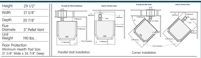
Tested by Warnock Hersey to UL 1482/ULC S627/CSA B366.2/ASTM E 1509-95. This pellet fired appliance has been tested and listed for use in maunfactured homes in accordance with Oregon Administrative Rules 814-23-900 through 814-23-909.
