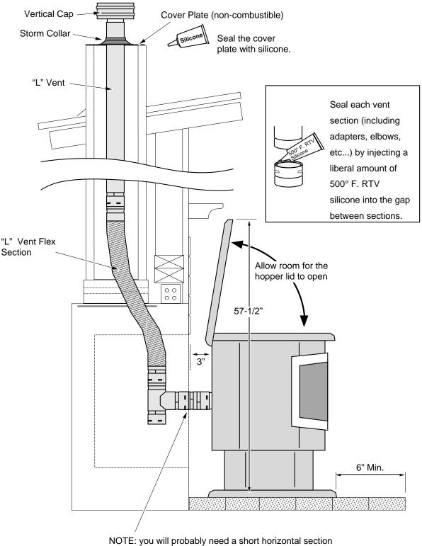
here to clear the lintel and allow the hopper lid to open.
