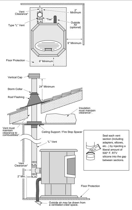
\* Install vent at clearance specified by the vent manufacturer.
