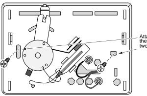
Attach the thermostat to the wall through these two holes.
