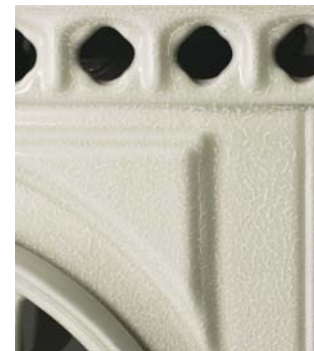
Porcelain Enamel Cracked Finish Detail
