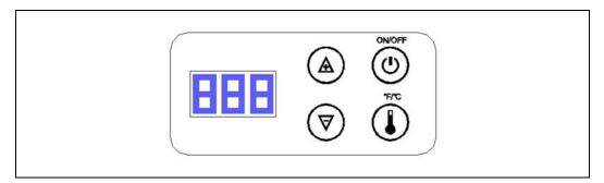
You can select temperature display setting from Fahrenheit to Celsius degree by pushing the **°F/°C** button/mark. Fahrenheit or Celsius degrees indicator will appear in blue color in the temperature display window.
