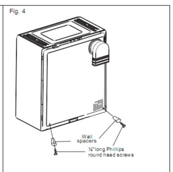
g) Mounting the dryer to the wall hanging assembly.
