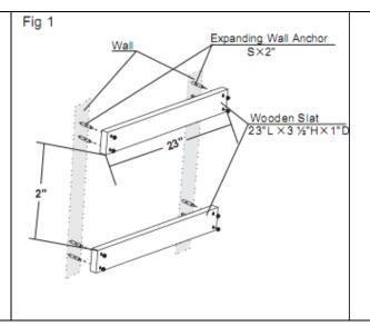
d) Install the wall mounting brackets to the wooden slats installed in the previous step.
