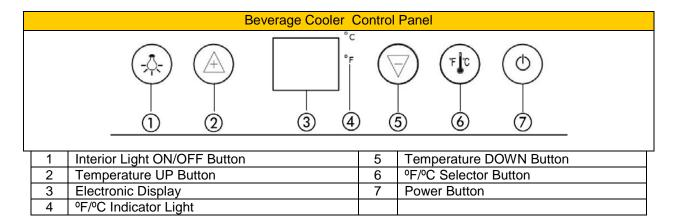
You can select temperature display setting from Fahrenheit to Celsius degree by pushing the °F/°C button/mark. Fahrenheit or Celsius degrees indicator will appear in green color in the temperature display window.
