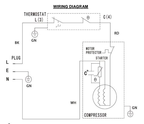
$\texttt{C}^{\texttt{*}}: \texttt{The capacitor is optional according to different compressor model}$
