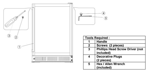
Install the handle with the two stainless screws provided with unit. Tighten the screws using a Phillips head screwdriver until the handle sets both flush and secured against the door frame. (DO NOT overtighten as this will cause damage to the handle assembly). See figure below.
