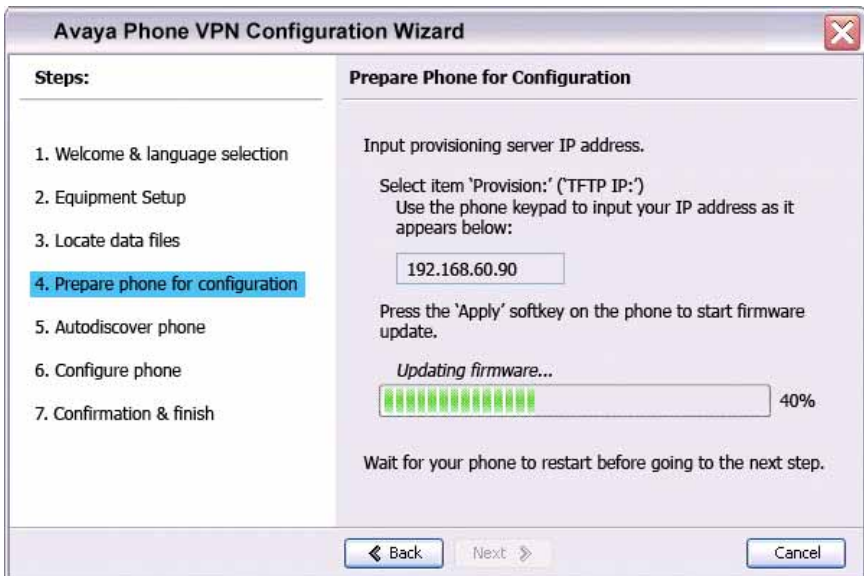
Figure 14: Prepare Phone for Configuration (Input Provisioning Server IP address )
