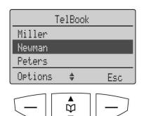
The 4 large keys below the display (see picture) are called the softkeys. The functions allocated to the keys are shown on the bottom line of the display. The key function changes automatically according to the telephone state.
