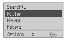
If the telephone book has been opened (\_\_\_\_-key), the arrow keys can be used to select a name and \_\_\_ or \_\_ can be used to dial.
