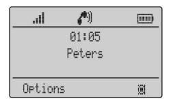
During a connection the loudspeaker volume can be adjusted by pressing the arrow keys.
