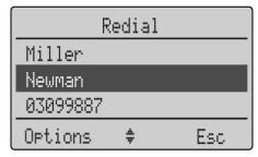
**Selection:** press the **(1)** -softkey and then one of the arrow keys with the telephone in an idle state. The last 10 phone numbers dialed are displayed. The beginning / end of the redial list is marked by a dashed line.
