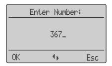
The arrow keys can be used to shift the input position (cursor) to the left or right. Additional characters are always added in front of the flashing cursor. Use **OK** to confirm your entry,  $\bigcirc$  deletes individual characters.
