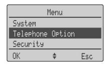
In this example, first press **Menu** and select **Telephone Option** with the arrow keys.
