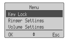
Press **Menu**. Use the arrow keys to scroll through this list and confirm the desired function with **OK**.
