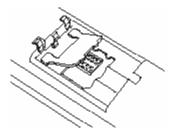
3. Press the memory card under the two teeth (a) so it slides into the memory card compartment. Make sure the contacts are face down as you do so and that the notched edge of the memory card is at the bottom left.
