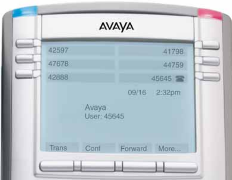
Figure 24: Logged in to an Avaya 1150E IP Deskphone
